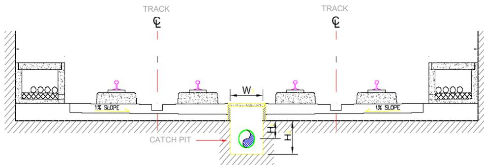
Figure 5. Example of typical drainage in tunnel
