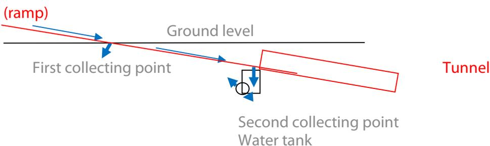
**Figure 4. Ramp to tunnel drainage principle**
